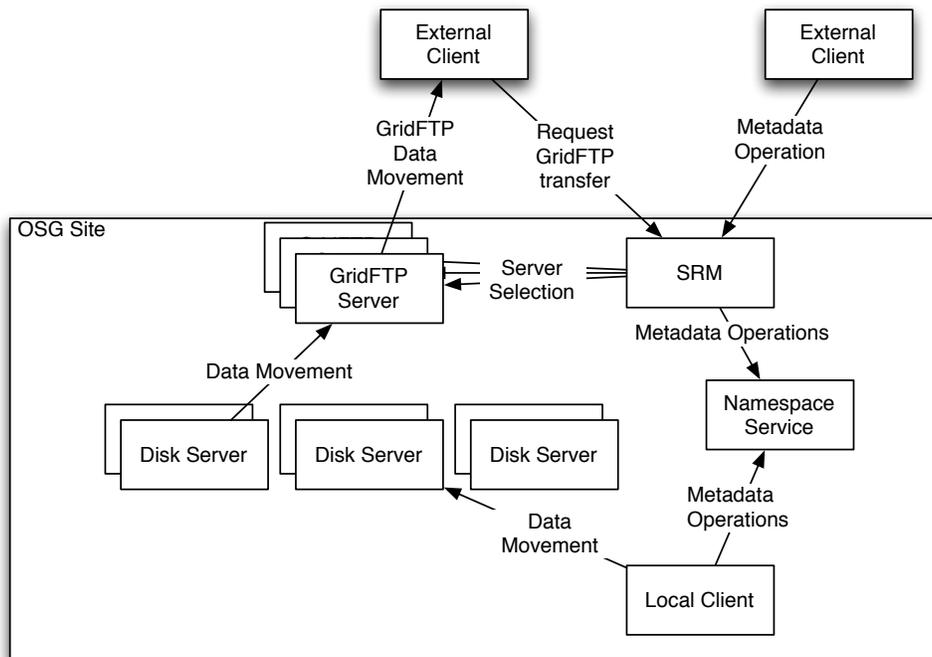
The OSG storage systems require files to be copied to the local site prior to the data being usable, a “push” model. For the LHC VOs, we support deploying HTTP proxies using Squid and allowing a “pull” model. This is limited to smaller files and unauthenticated access. For authenticated, large-scale data movement using the “pull” model, we are investigating the Xrootd software.
